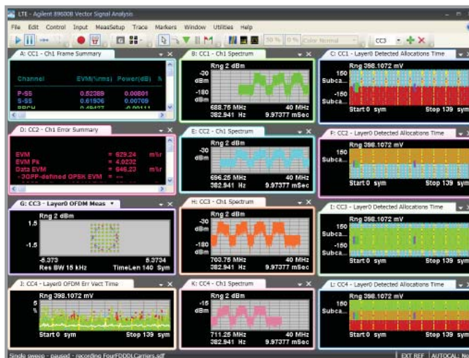
Fully characterize up to 5 CCs -- simultaneously. Set up the measurement parameters and view different measurements on each.
