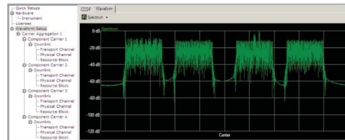
Spectrum of LTE-Advanced configuration with four 20 MHz component carriers
